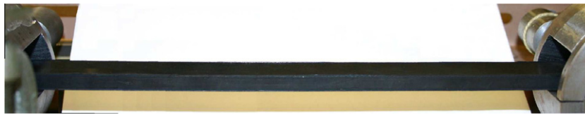
Fig. 2. Principal solution of the fiber-reinforced rubber slab bonded on a thin metal plate and subjected to pure bending. (Photo courtesy of Astier and Caillard (2006)).
