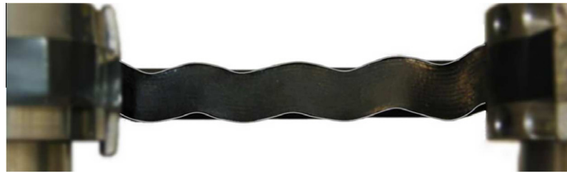
Fig. 3. Buckled state of the fiber-reinforced rubber slab bonded on a thin metal plate and subjected to pure bending. (Photo courtesy of Astier and Caillard (2006)).
