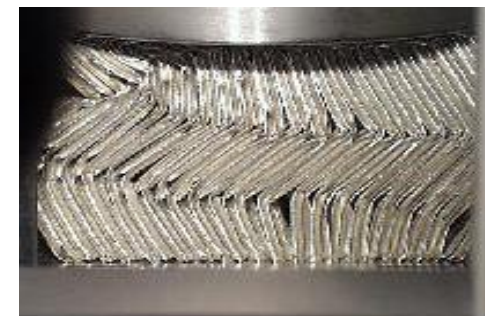
Failure mechanism at 165 °F
