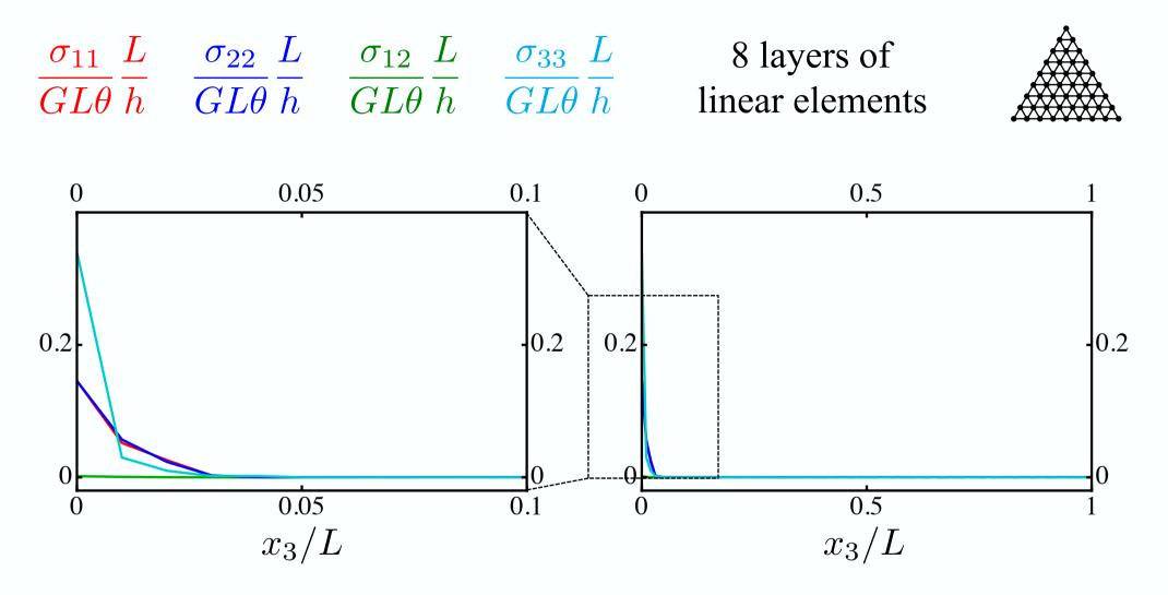
Since warping in prevented at  $x_3=0$ , normal (and a tiny in-plane shear) stresses develop in a boundary layer of the order of the section thickness
