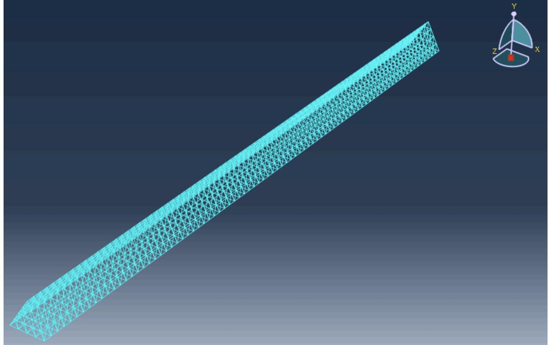
NOTE on meshing: a straightforward division of the pentahedral prism in three tetrahedra gives one ill-conditioned element; as a result the code automatically changes meshes to have well-behaved elements (with gradients of the same order in all directions). This explains the rather bizzare number of total elements in the 3D prism
