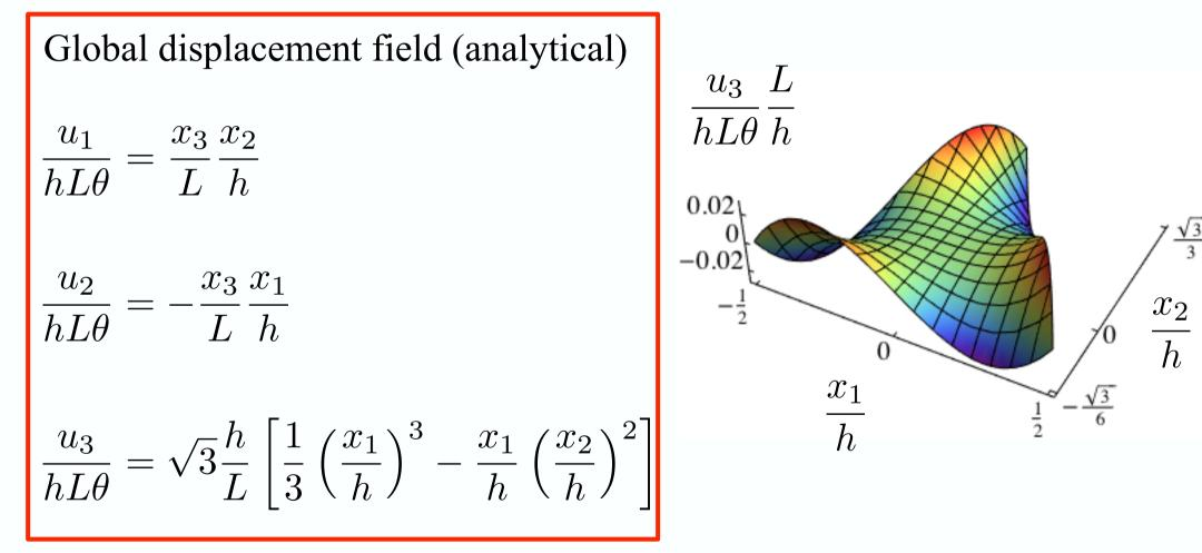
Notice the  $C_3$  symmetry of the warping (i.e.  $u_3(x_1, x_2)$ ) distribution; Warping is zero at middle of the section and of the edges
