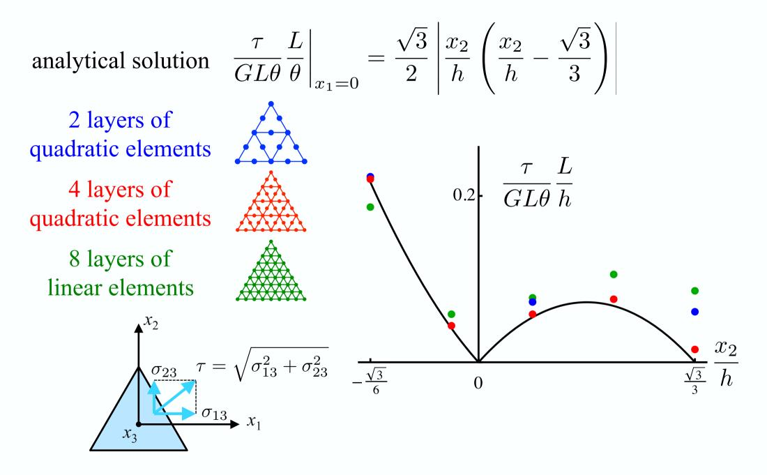
**TORSION OF A TRIANGULAR SECTION BAR CLAMPED AT**  $x_3 = 0$
