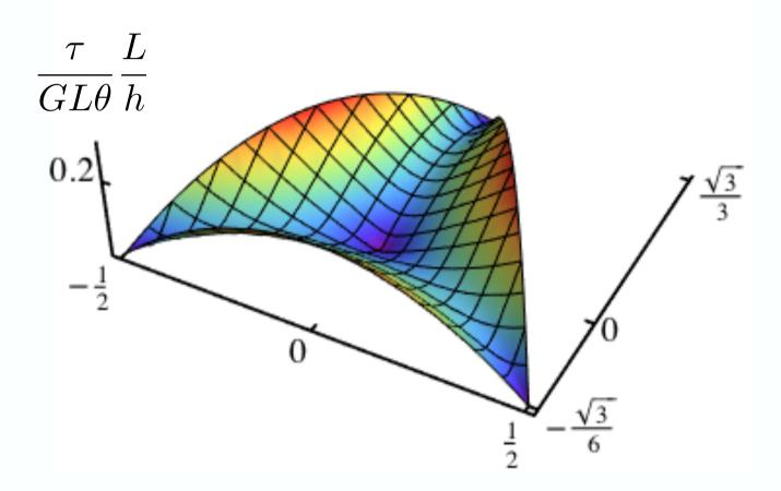
Notice the  $C_3$  symmetry of the stress distribution; Stress is zero at middle and at corners and maximum at middle of edges
