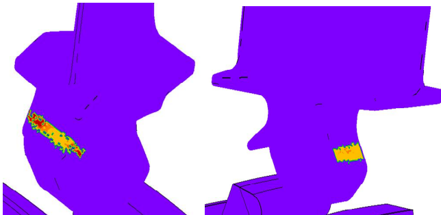
Figure 15 – Friction Coefficient distribution on blade contact surfaces
