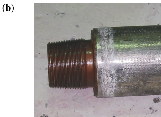
Fig. 1. Description of a drillstring: (a) drillstring components and (b) picture of the pin part of a tool-joint.
