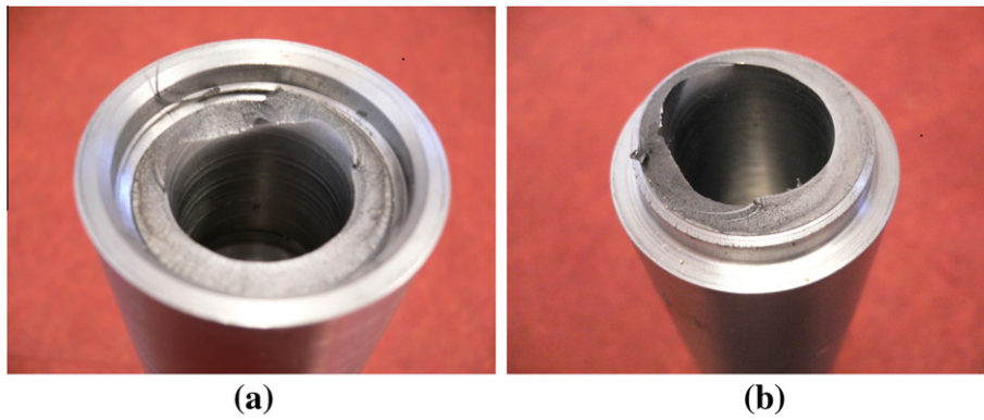
Fig. 11. Photographies of the downsized threaded connection after failure: (a) box and (b) pin.
