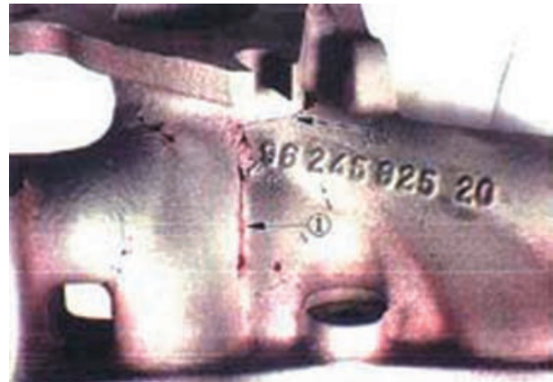
Fig. 9 Results of an engine bench test: cracked area observed on the prototype.
