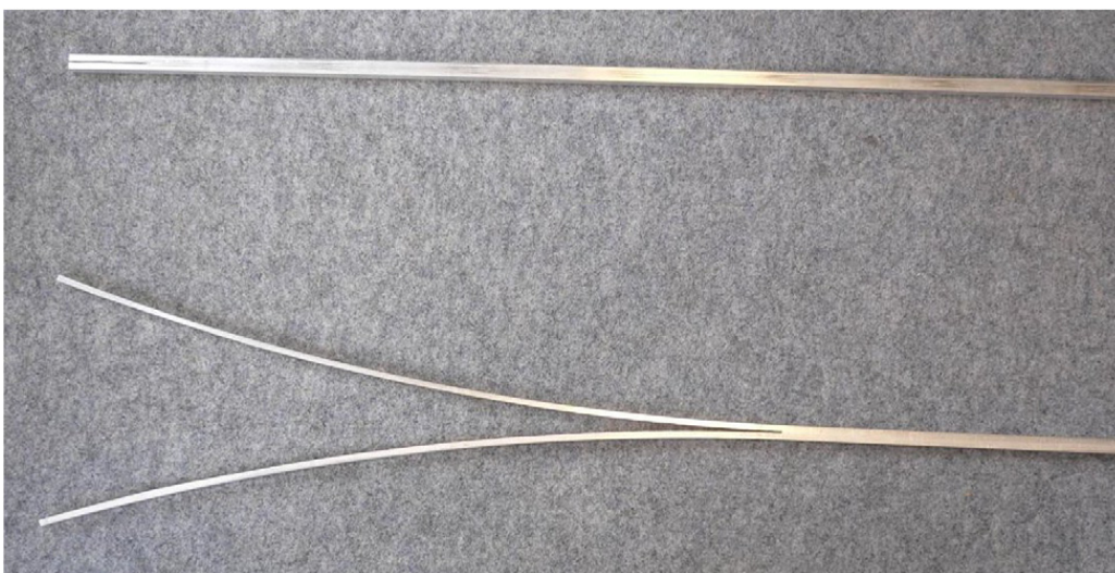
Fig. 1. Deformation of an aluminium rod after cutting, due to the presence of residual stresses, an experiment proposed by Prof. H.D. Bui.
